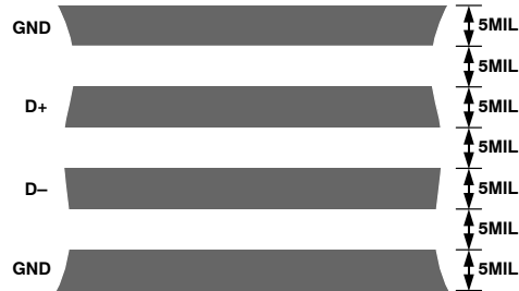
Figure 16. Arrangements of Signal Tracks
